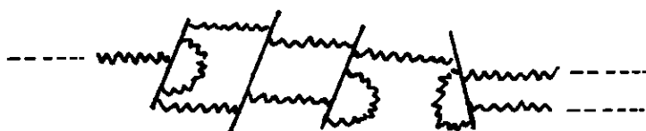
Fig. 5 A schematic presentation of structure of [-AB_m]_n segments copolymers
